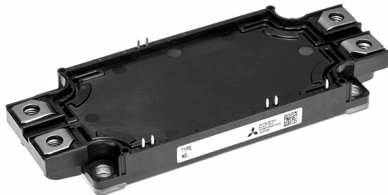
Dual switch (Half-Bridge)
